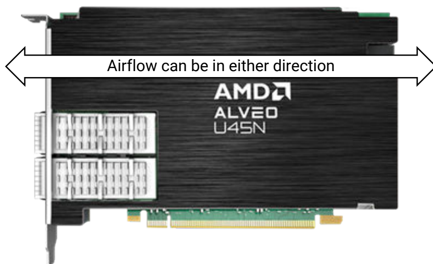
Figure 6: Airflow Direction for U45N Accelerator Card
